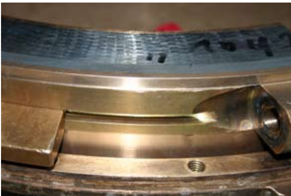
Figure 4 The Babbitt bearing after the two months field test.
