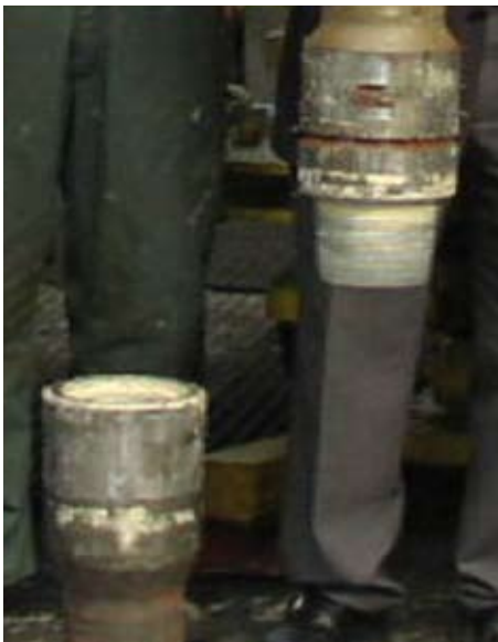
Figure 5 Connection after break-out
