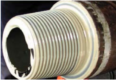
Figure 4 Drill pipe after first break-out
